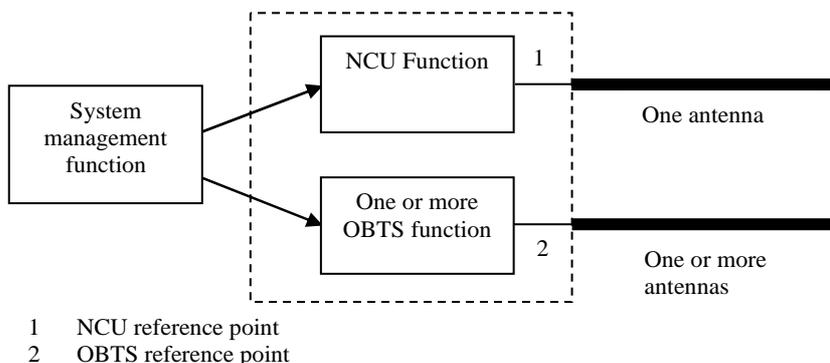
**Figure 5.2.0-2: MCOBA System reference points without antenna coupler**
