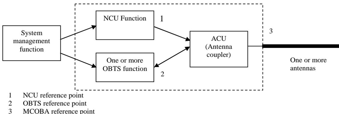
NOTE: The system reference points in this figure show the antenna coupler as separate functional block. It should be noted that the antenna coupler functionality can be integrated in the NCU functional block as well as the OBTS functional block as well. This does however not affect the definition of the measurement reference points above.
